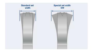
Special set width SW: The extra wide set achieves the free cut of the band saw blade so that there is more clearance to prevent jamming due to decreasing material residual stress.
