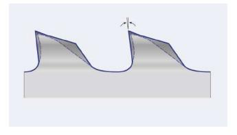
About the profile tooth form: The tooth features a positive cutting angle and a reinforced tooth back.
